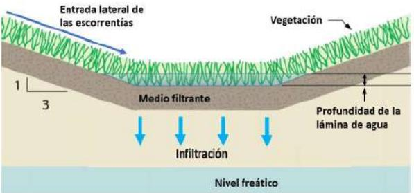
Figura 71 Esquema de una cuneta vegetada. Fuente: Adaptado de New Jersey Department of Environmental Protection Division of Watershed Management (2021).
